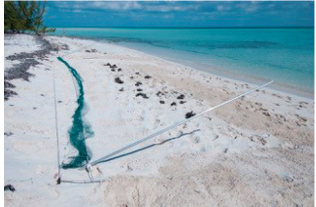
A bungee-powered net used to capture roosting Piping Plovers. When the net is triggered, it moves quickly up and over a group of birds resting among the clumps of wrack (the dark spots in the sand). Flag 5C and 3T were captured in the same roost in the Joulter Cays north of Andros, Bahamas. Photo by Walker Golder.
